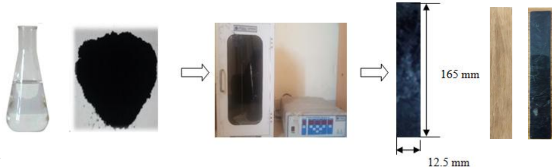
Figure 1. Nano composite specimen preparation and nano, sisal and hybrid composite
